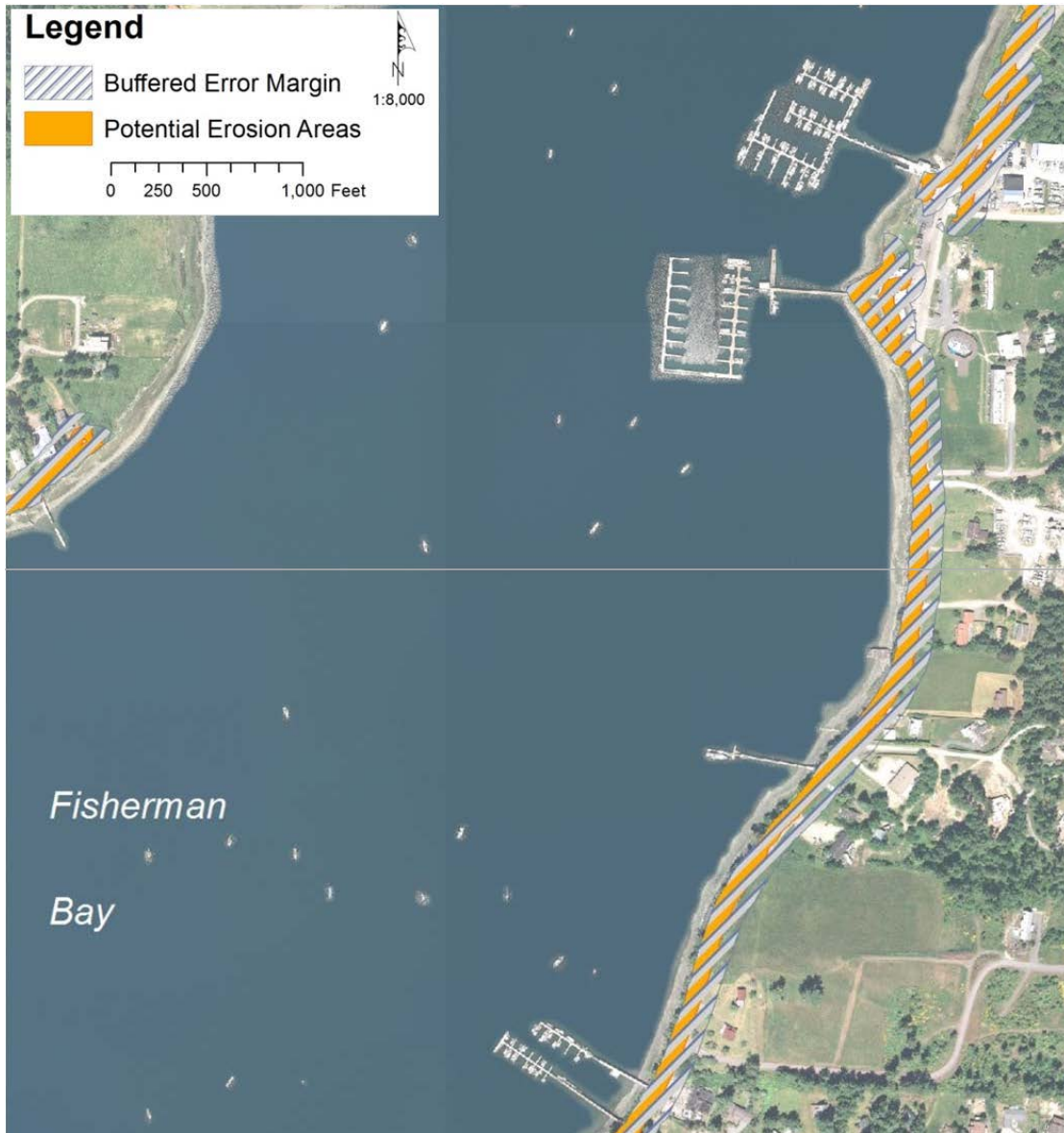
Figure 17. Example of buffered error margins to erosion vulnerability for the high SLR scenario in 2100 for Fisherman's Bay, Lopez Island, as found in project GIS geodatabase to facilitate communicating uncertainty in outreach efforts.
